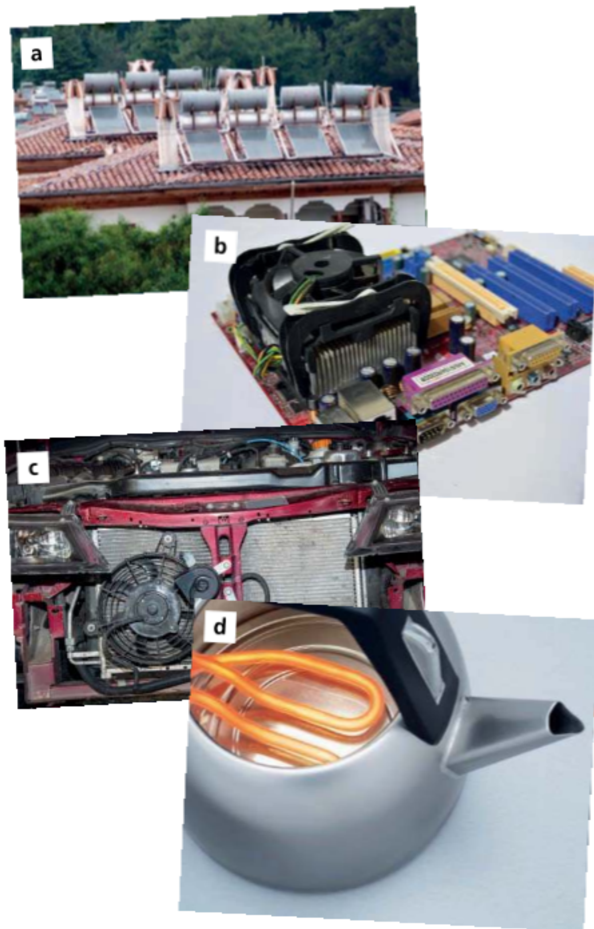
■ Figure 4.17 (a) Water heating solar panels, (b) a 'heat sink' on a microprocessor in a computer, (c) the radiator on a car engine (d) an electric kettle heating element
